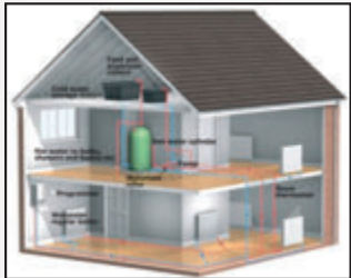
Conventional Heating System
